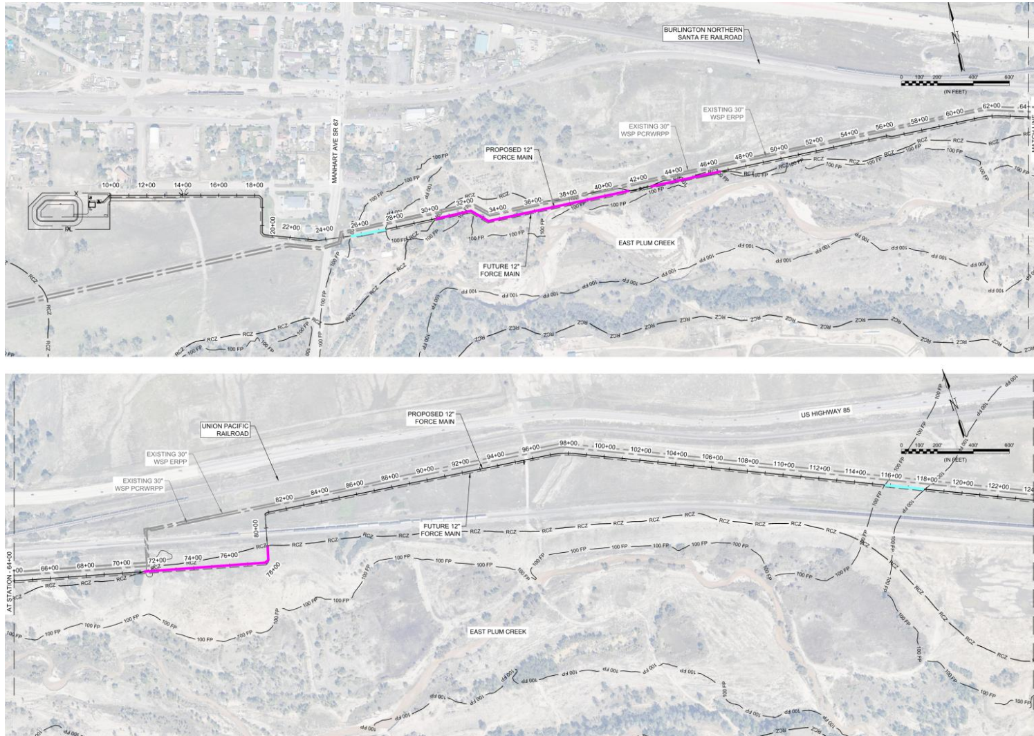
Figure 1-2: Open Cut Installation in 100-yr Floodplain (Cyan) and RCZ (Magenta)
