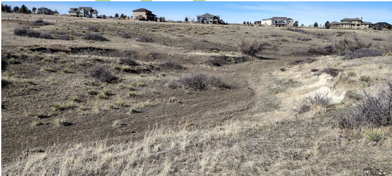
PHOTO 4. Downstream end of Tallman. Only a small defined drainage path was observed with the base of the generally wide drainage stable and vegetated. Signs of past bank erosion are observed, but steeper slopes have revegetated indicating limited active erosion. Overall, the channel was observed to be erodible but stable.
