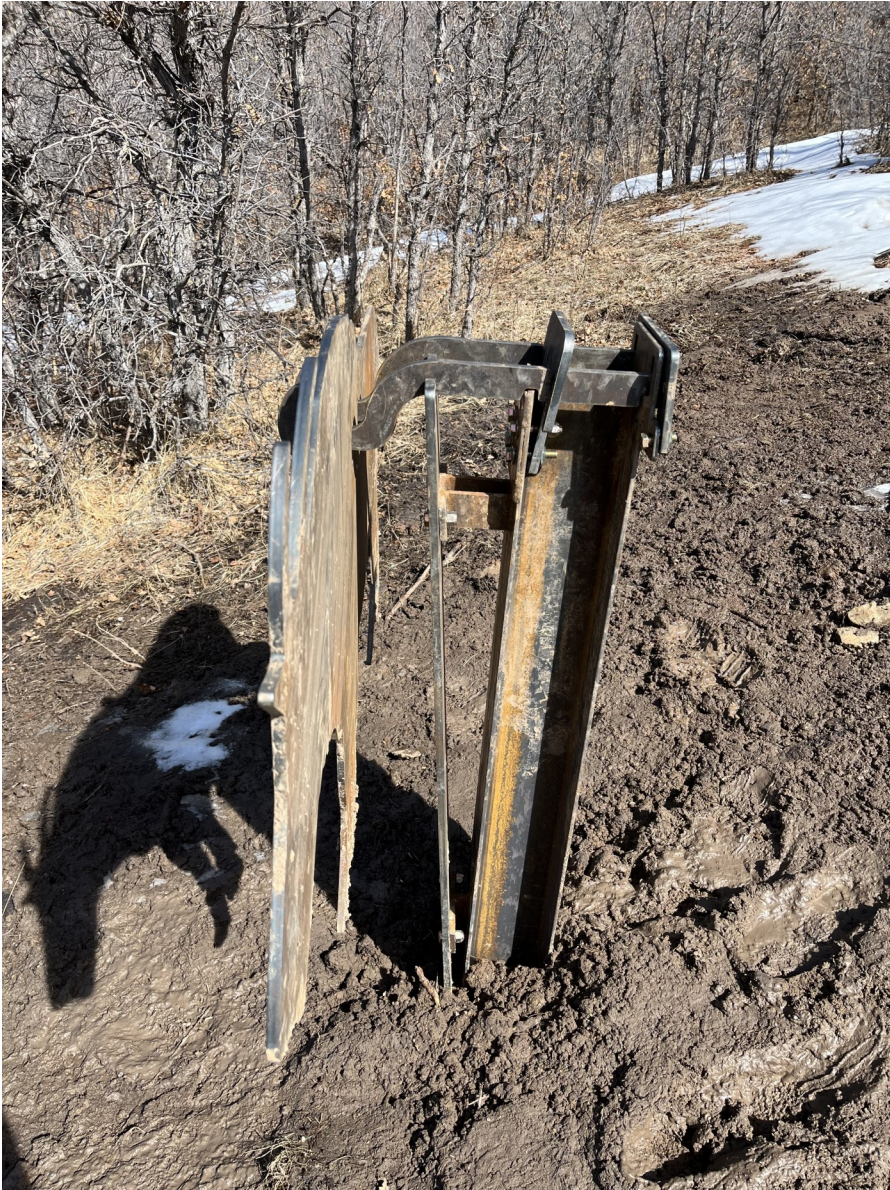
Target stand and hanger system. Mounted onto concrete block base.
